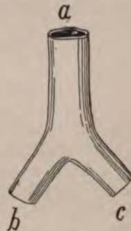
FIG. 47.—If a vessel (a) divides into two branches, (b) and (c), these will be individually of less cross-section than the main trunk but unitedly they will exceed it. Linear velocity will be lower in the branches than in the parent stock.
